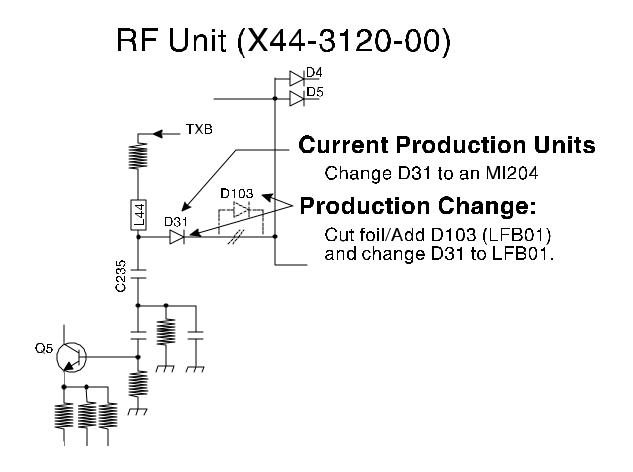
**Caution:** This modification requires soldering equipment rated for CMOS type circuits. It also requires familiarity with surface mount soldering techniques. If you do not have the proper equipment or knowledge do not attempt this modification yourself. Seek qualified assistance.
