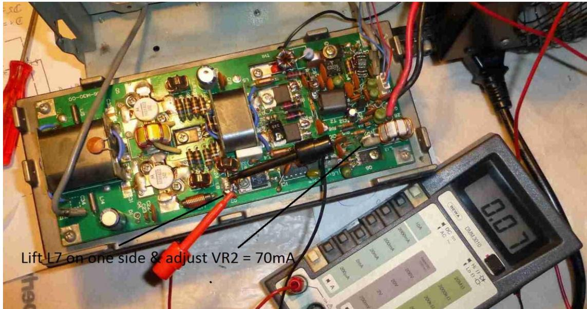
Note how Marcel lifted the side of L7 near the regulator to set the idle current. Extreme care needs to be taken here not to short anything out.. The main idle current measurement shown below is much easier.
